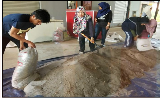
Figure 3.2 : Process of mixing and sieving BRIS soil.
