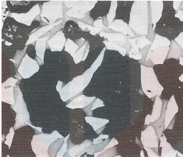
Figure 2.4 : Photomicrograph of an \text{Al}_2\text{O}_3 bonded ceramic abrasive grains (Callister, 2011)
