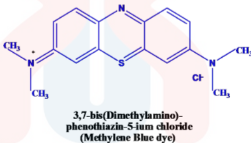
Figure 2.2: Methylene blue chemical structure with its systematic (IUPAC) name. (Source: Thakur et. al , 2016).
