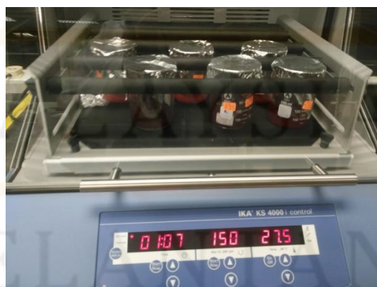
Figure C.2: The solutions were stirred at constant speed of 150 rpm at ambient temperature for 120 minutes.
