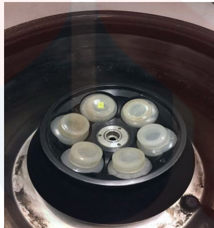
Figure 3.4: GO were put in the centrifuge tube. The mixture were equally divide into 6 centrifuge bottles. The mass of the mixture were ensure to be balanced before the centrifuge were run.
