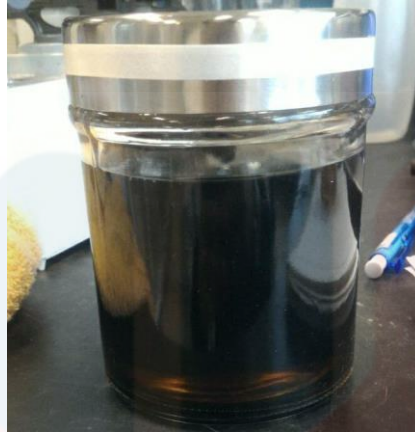
Figure 3.6: GO Gel were obtained after being dried under vacuum.
