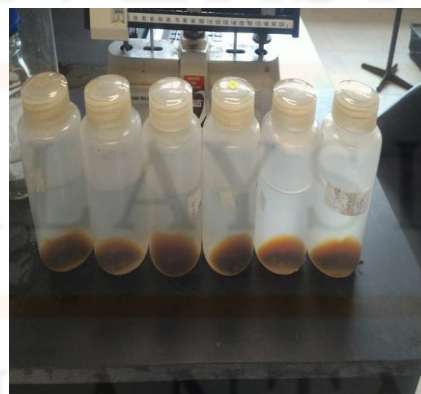
Figure 3.5: GO mixture after being washed for 4 times.
