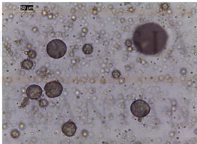
Figure 4.9: PMMA-co-MAA hollow colloidosomes rotary evaporated at 8 mins Leica image
