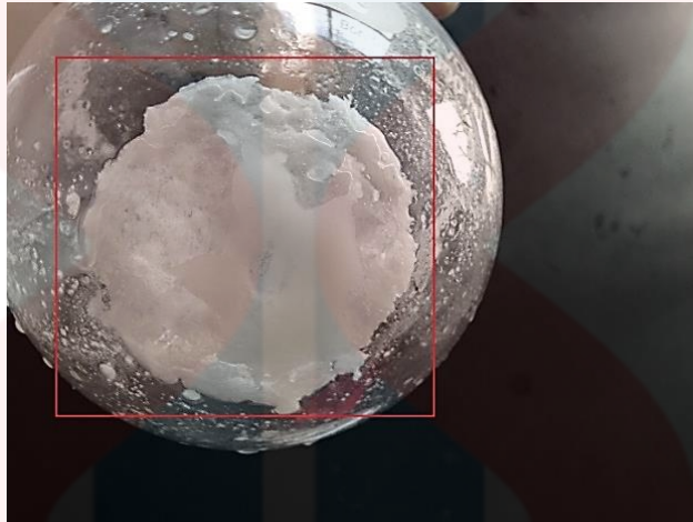
Figure 4.8: PMMA-co-MAA sample aggregated in 10 mins' rotary evaporation
