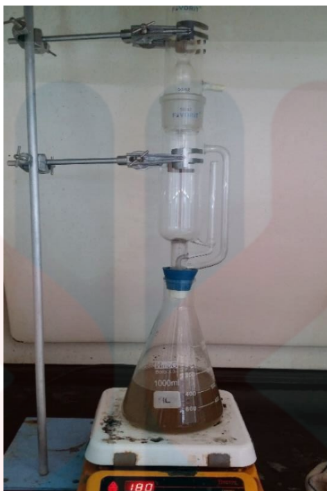
Figure 3.6: Soxhlet set up for lignin extraction
