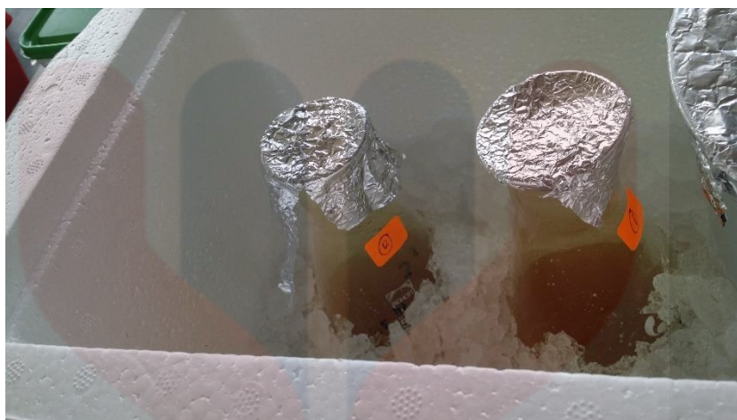
Figure 3.5: Colling process for holocellulose extraction process
