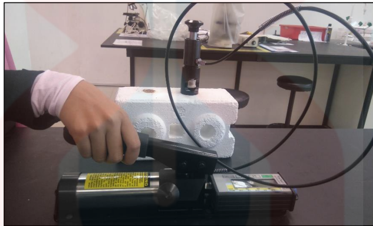
Figure 3.12: Determination of coating adhesiveness
