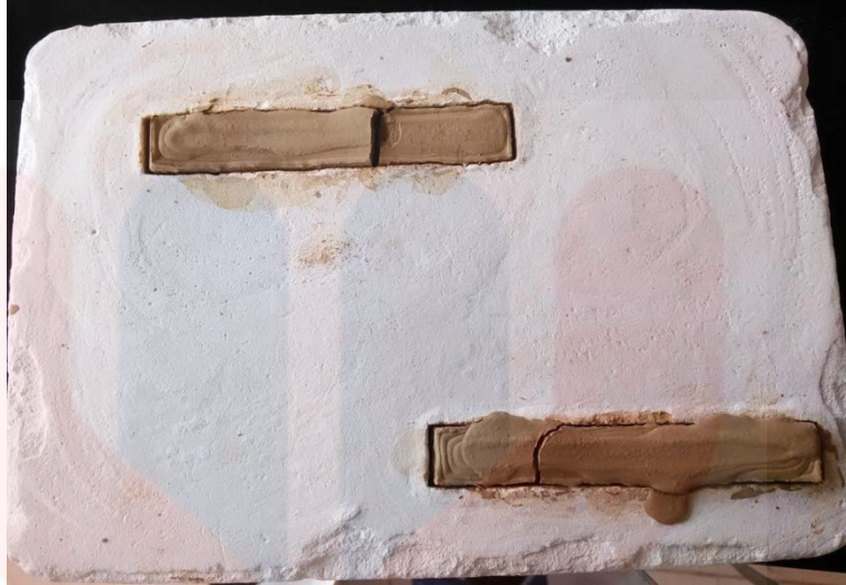
Figure 4.2 Crack present in green body of 50C50W due to present of too much water contents
