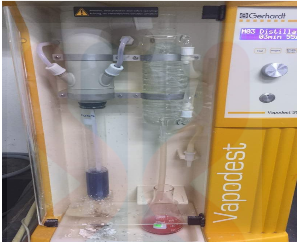
Figure A.11: Distillation process of crude protein
