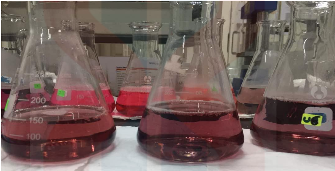
Figure 3.1: After titration process, samples turns to greyish pink.
