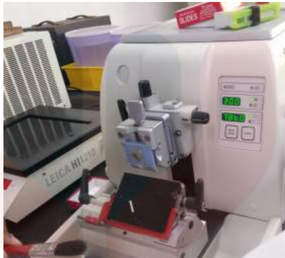
Figure A.5 Trimming process to remove excess paraffin from cassettes using microtome.
