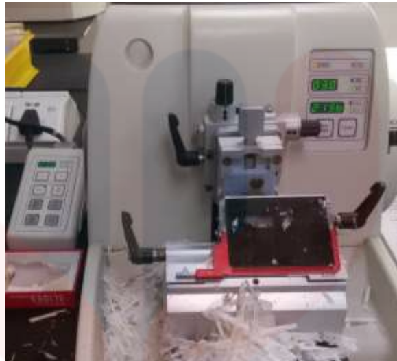
Figure A.7 Process sectioning tissue use microtome
