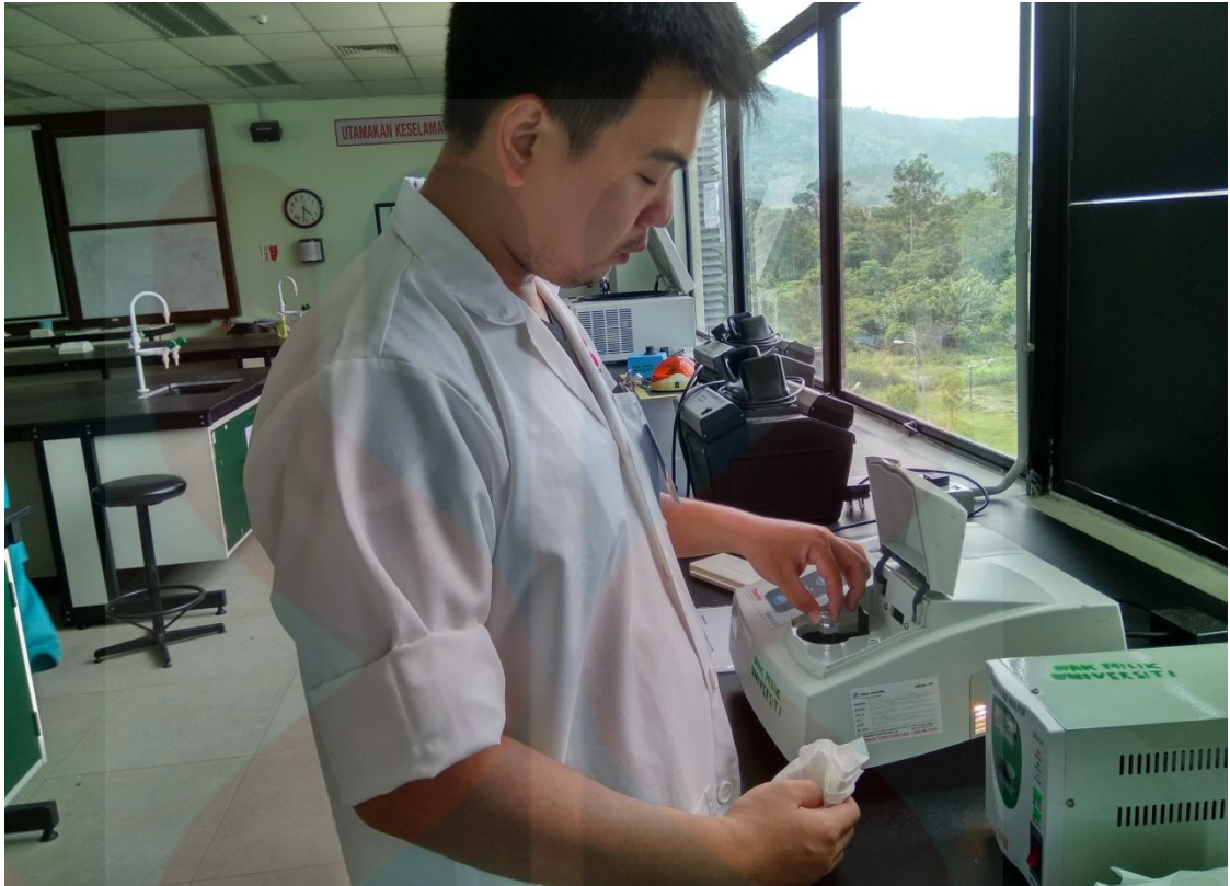
Figure B.7 : Checking OD reading using spectrophotometer.
