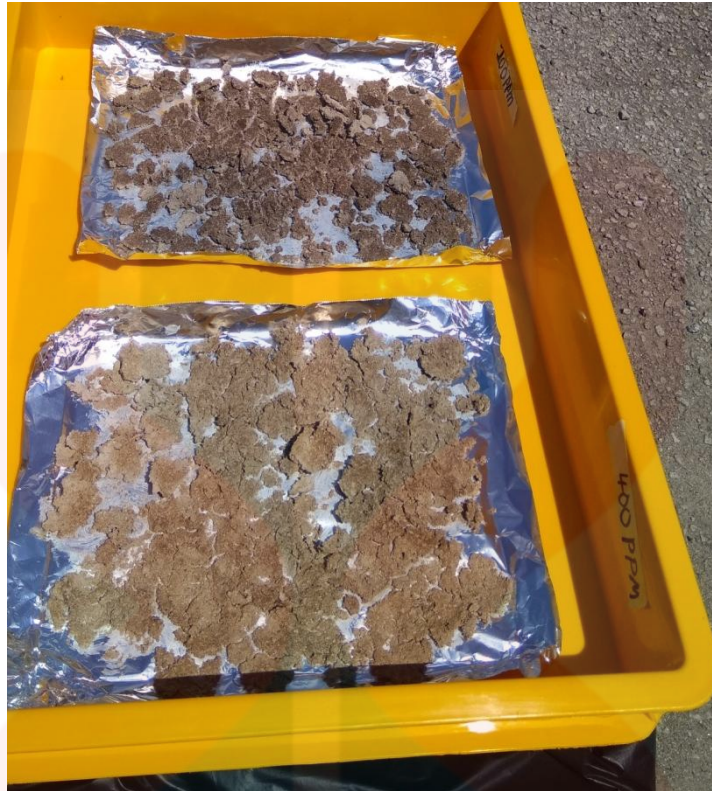
Figure B.3 : Drying of TQD under sunlight for 24 - 48 h.
