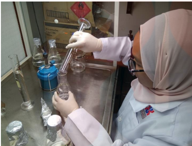
Figure B.4: Distilled water ( \text{dH}_2\text{O} ) were autoclaved were put into the 400 mL of conical flask.
