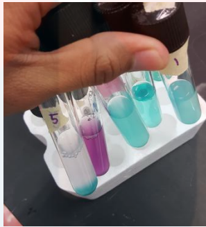
Plate II : Nitrite result of EBN supernatant samples for EBN natural habitat (cave) and modified habitat (house) by commercials kits (Nitrite water test kit).
