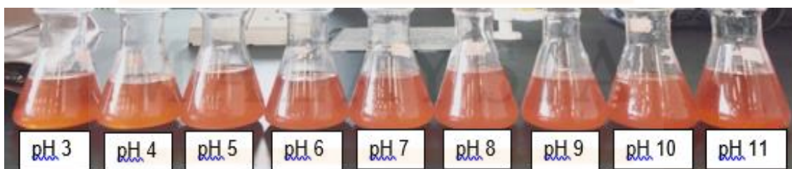
Figure B6(i): MO dye in different pH solution with adsorbent after 3 hours
