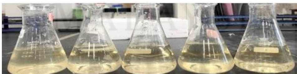
Figure B9: The colour changes of MO dye after going through membrane filtration
