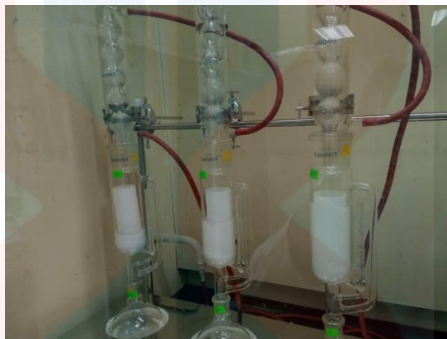
Figure 4.1: Fat extraction process using soxhlet extraction (Sources: © Umi Raihanah 2018)
