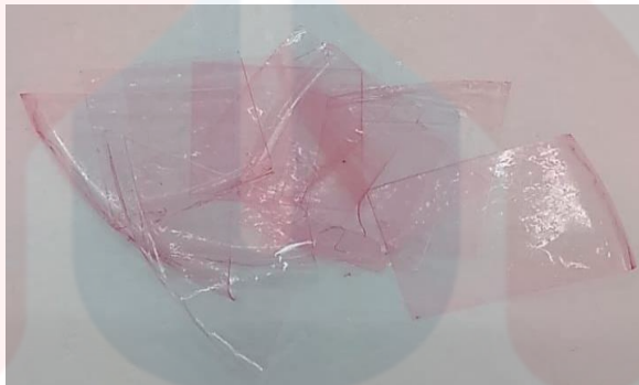
Figure 11 : CTA PIM with 50 wt. % Aliquat 336 after extract under optimized condition (2 ppm of Congo red, Congo red in pH 2, 30°C and 150 rpm)
