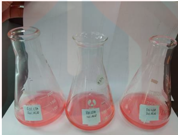
Figure 8 : Congo red before extraction which contain CTA PIMs with 40%, 30% and 20% of Aliquat 336 in pH neutral.
