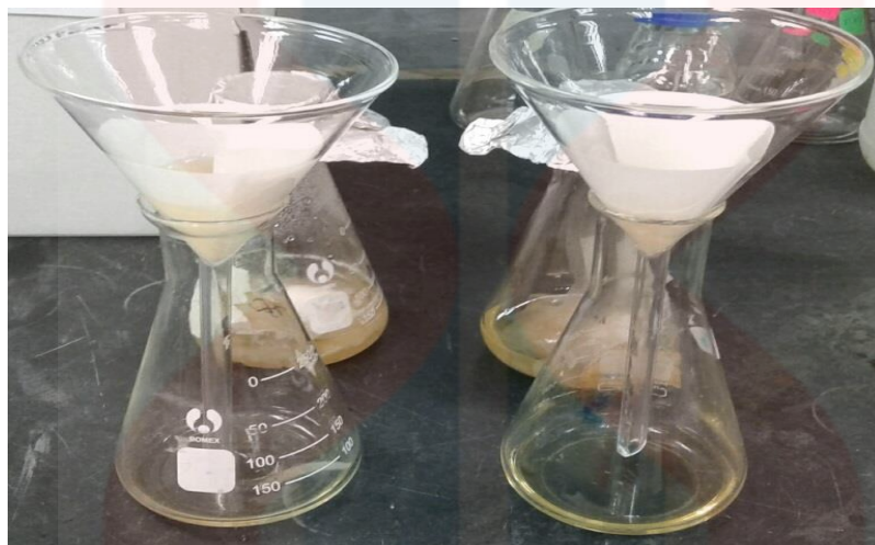
Figure 3.1 The filtering process of UMKRSPL1 culture with Whattman filter paper No. 1
