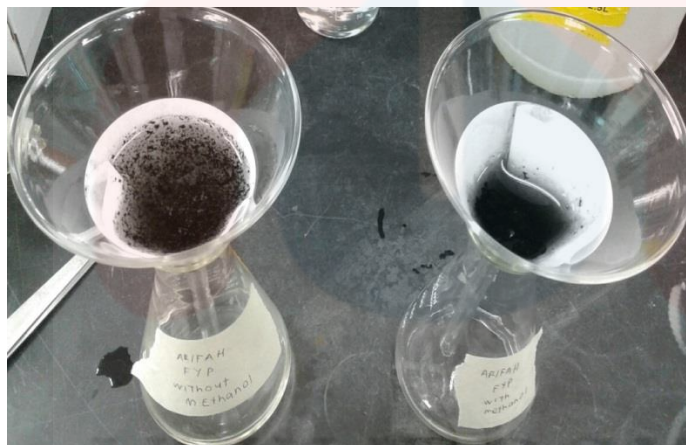
Figure 3.7 Filtration of charcoal-treated solution with filter paper
