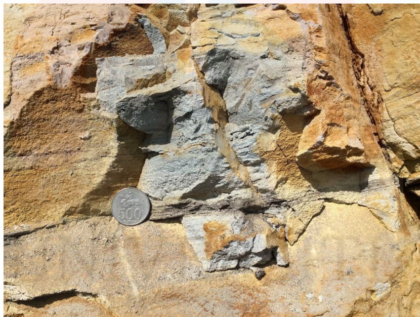
Figure 5.3.1 b: Massive volcanic sandstone with medium to coarse grain with parallel lamination
