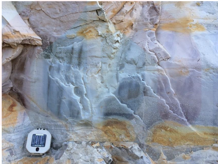
Figure 5.3.5 c: Very fine tuff present in compact and hard and some parallel lamination near compass
