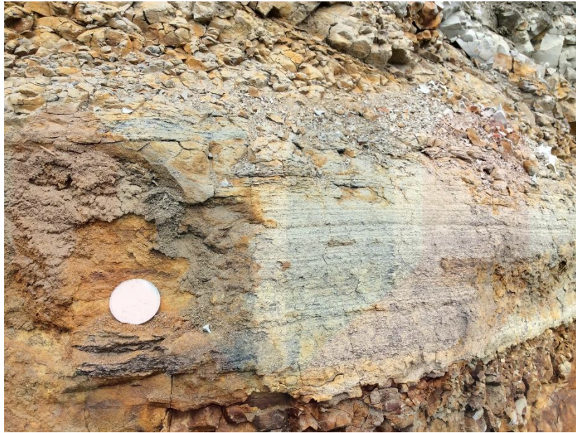
Figure 5.3.1 a: Siltstone laminated mudstone with carbonaceous claystone
