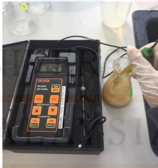
Figure 3.2: Tested soil's pH by using pH meter.
