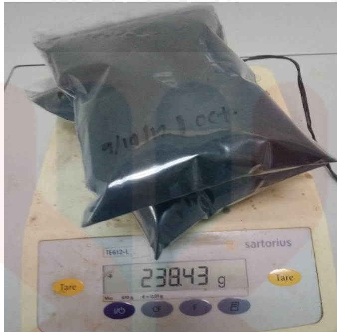
Figure 3.11: The weight of activated carbon after furnace under 800°C for 6 hours.
