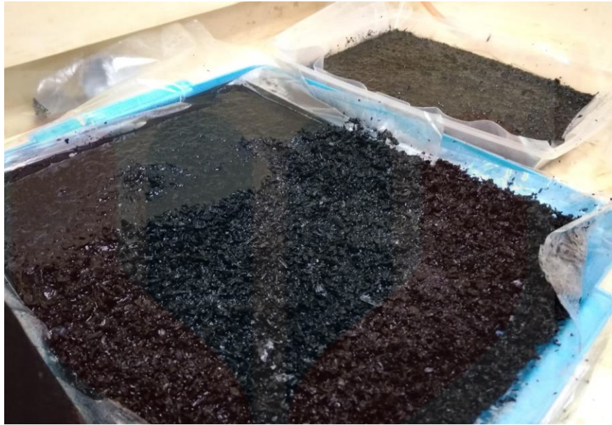
Figure 3.5: Well soaked active carbon is filtered and left in the hood for few days to dry completely.
