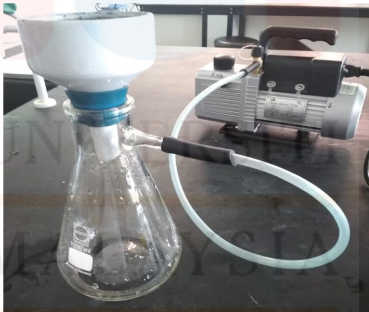
Figure 3.12: The vacuum pump is used with filter paper to wash the activated carbon.
