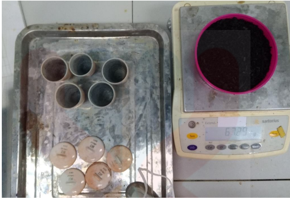
Figure 3.7: The weight of AC in 5 crucibles 67.29g before furnace.
