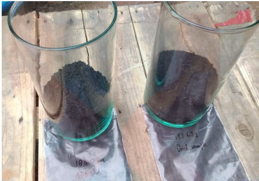
Figure 3.1: Charcoal before soaked with hydrochloric acid
