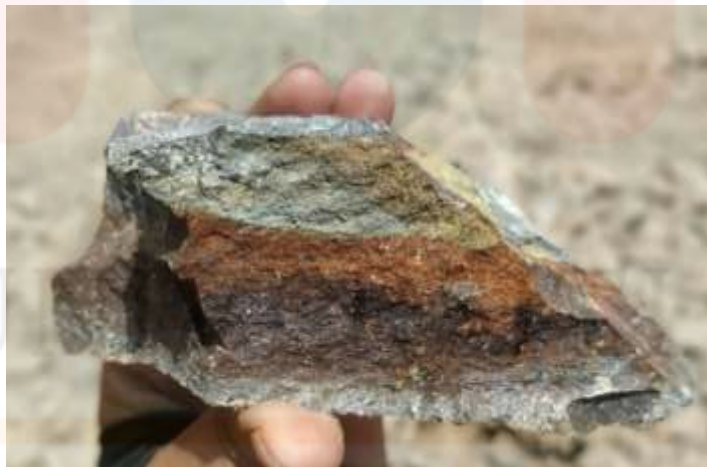
Figure 4.13 Rusting effect due to oxidation process
