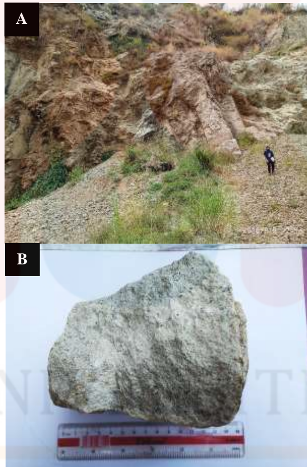
Figure 4.25 Tuff rock (A) Outcrop of tuff contact with andesite (B) Hand specimen of tuff
