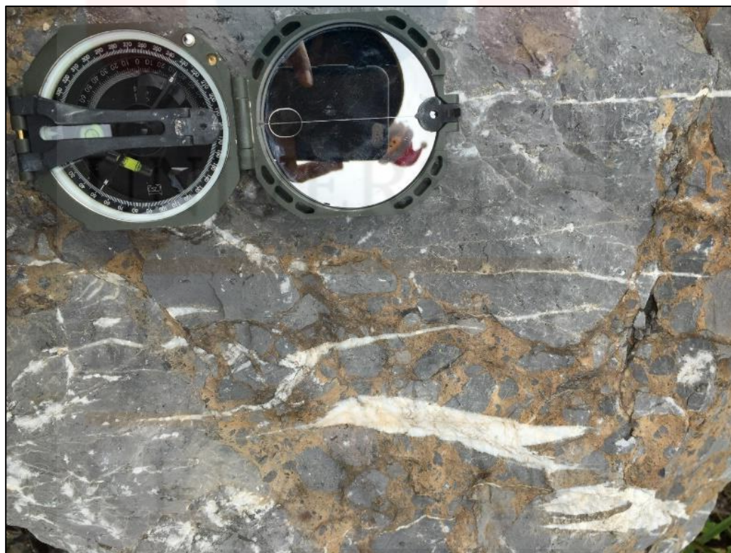
Figure 4.40: Calcite vein at a limestone rocks which reacts vigorously with hydrochloric acid (HCL)
