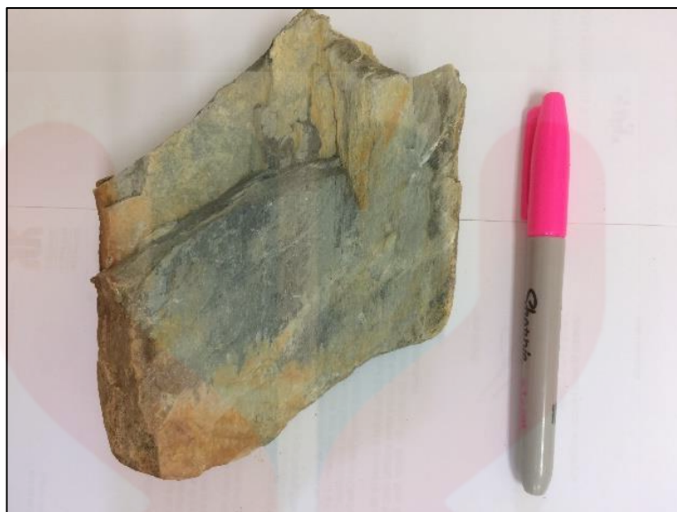
Figure 4.25: Hand specimen of shale rock sample.
