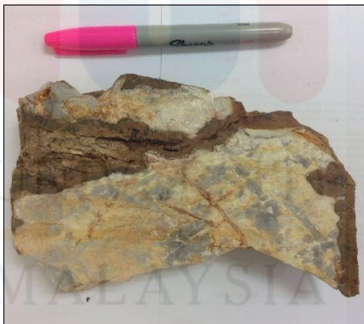
Figure 4.31: Hand specimen of chert rock sample.
