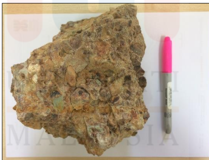
Figure 4.22: Hand specimen of conglomerate breccia rock sample.
