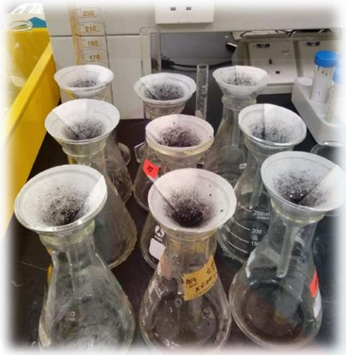
Figure 9: Filtration of extraction.
