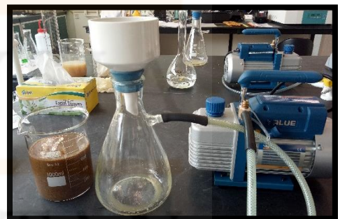
B.6: The solution has been filtered using vacuum pump.
