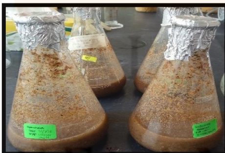
B.5: Treated pineapple peels after stir using rotary shaker.
