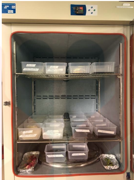
Figure B.3: The drying process of gelatin solution inside drying oven at 45°C until the samples were dried completely.
