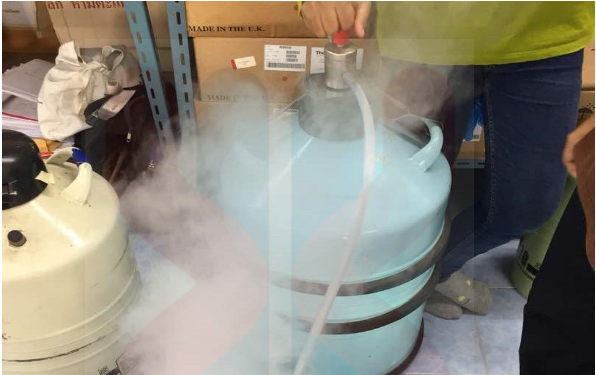
Figure B.9 Liquid nitrogen tank at -198^{\circ}\text{C} for freezing semen treatments storage
