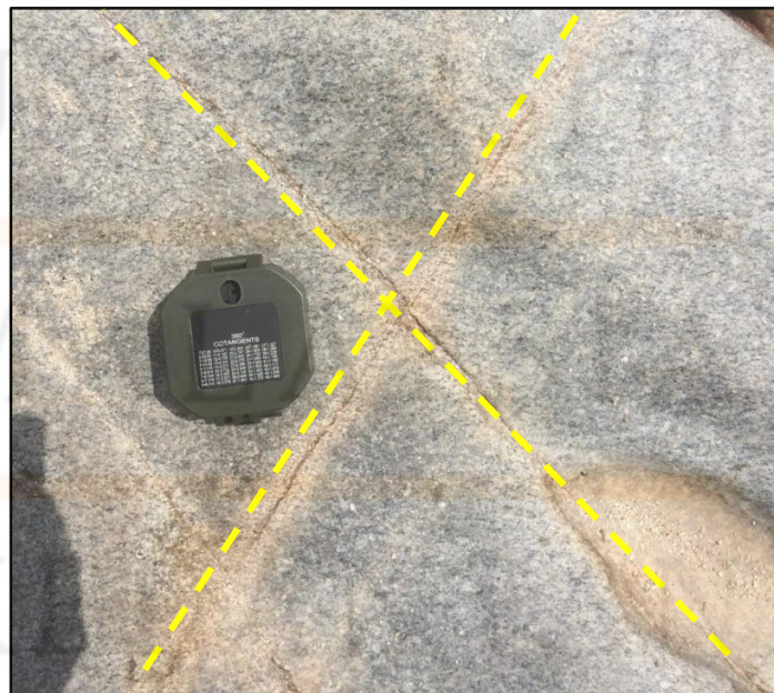
Figure 4.23. Conjugate joint structure (yellow dashed lines) of granite body at Sungai Terang.
