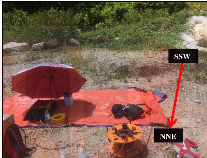
Figure 5.5. Set-up for center of spread Survey Line 1.
