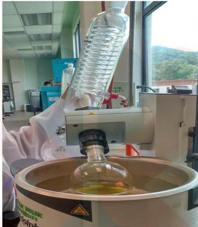
Figure 5.3 : Removing solvent using Rotary evaporator
