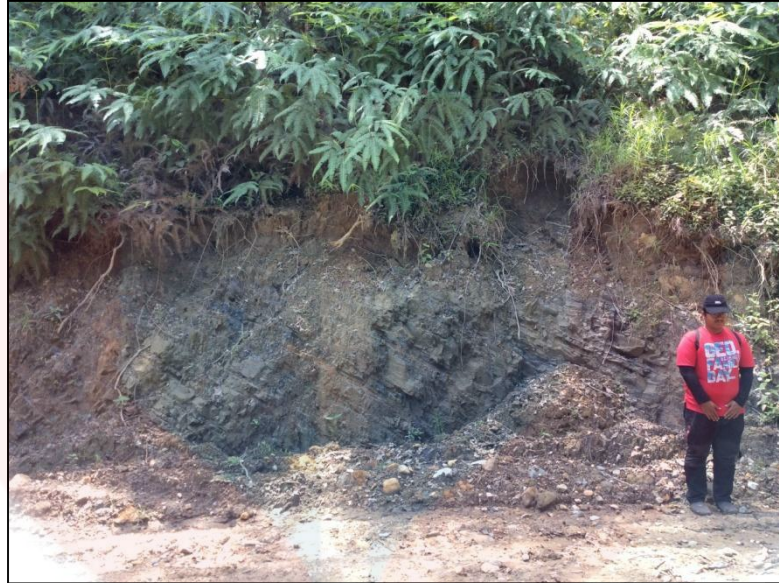
Figure 4.19: Physical weathering that undergo by slate rock with grade IV ( highly weathered)
