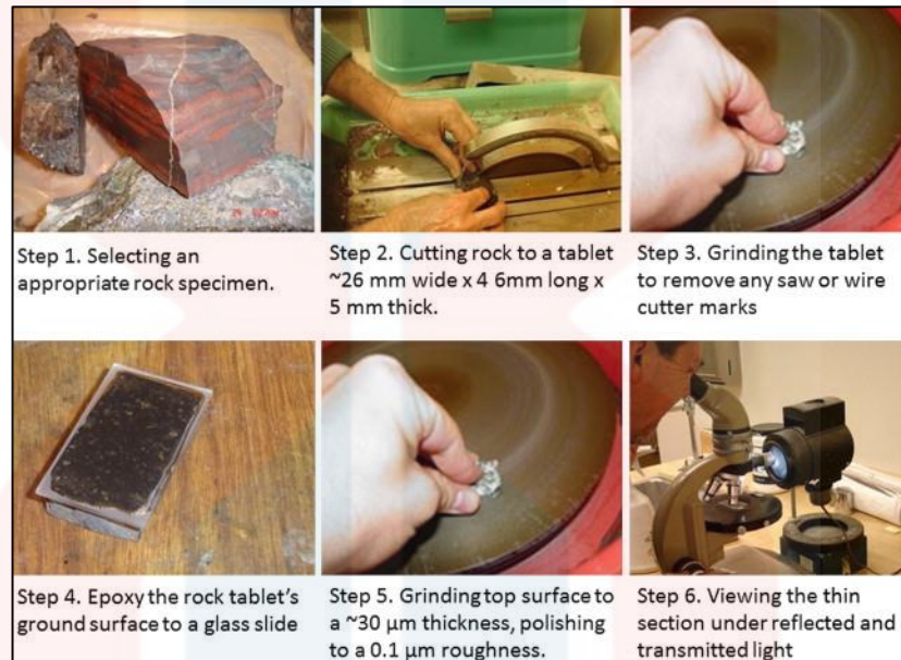
Figure 3.3: steps for thin section preparation (source: Gale et, al , 2013)
