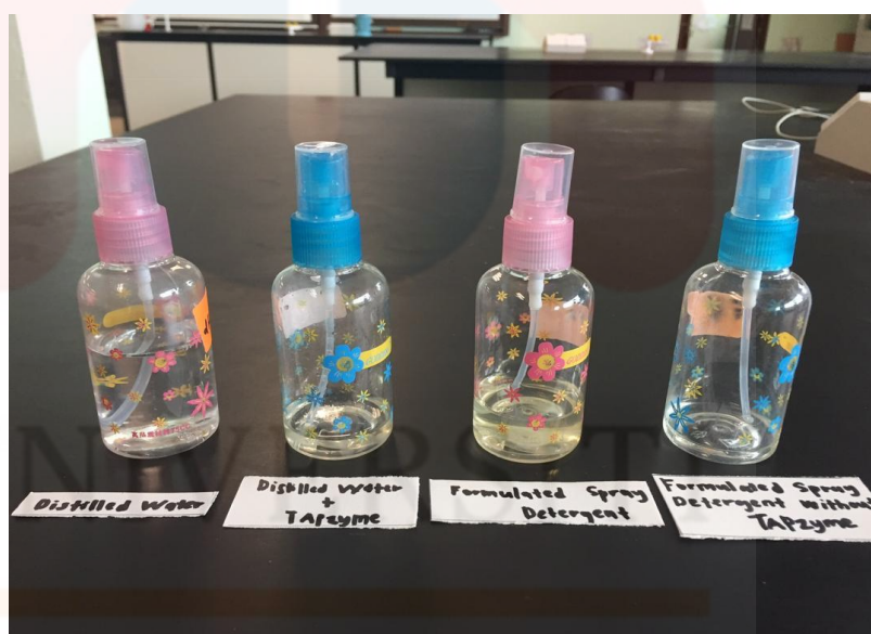
Figure 4.2: Four types of removal bloodstains were sprayed with 300 \mu\text{L} at 5 cm from the spray bottles to the fabrics
