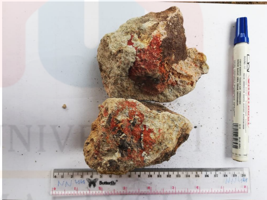
Figure 4.27: Hand specimen of volcanic breccia's matrix in NN24. The matrix is made up of tuff, highly weathered.
