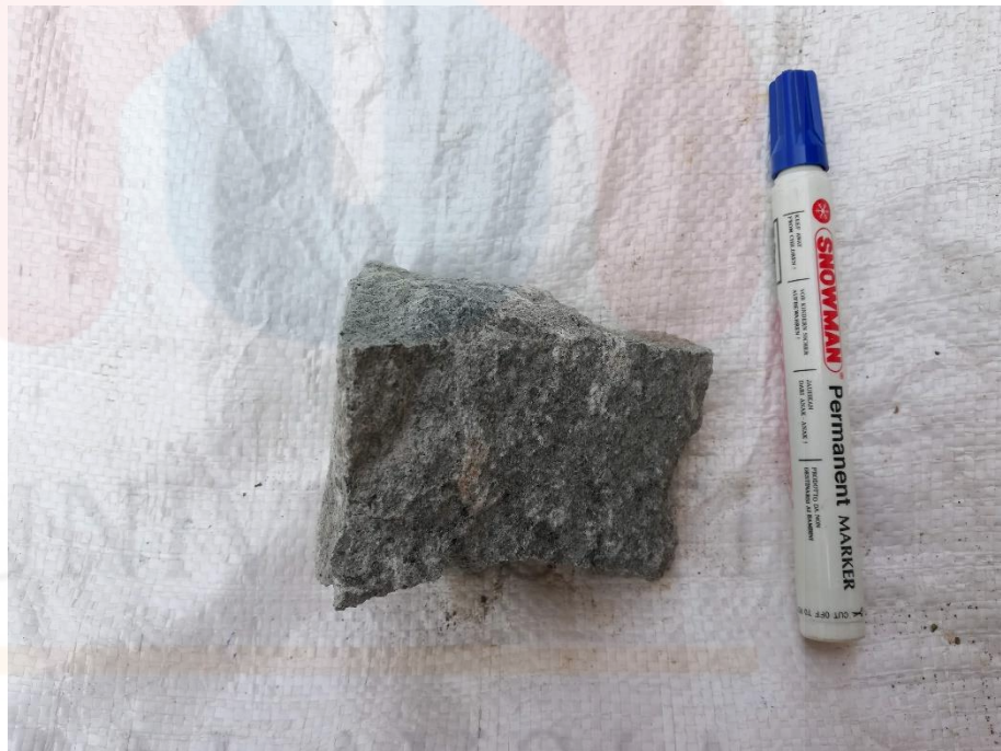
Figure 4.20: Hand specimen of pyroxene andesite in station NN1.
