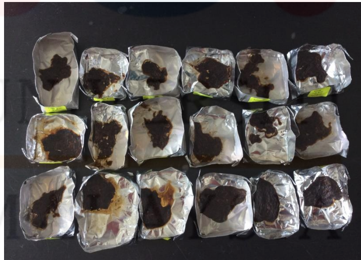
Figure 3.3: Dry tissue that has been kept in an air-circulation oven for 24 hours
