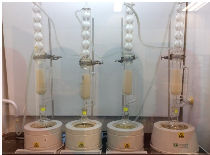
Figure 3.5: The set-up of soxhlet apparatus
