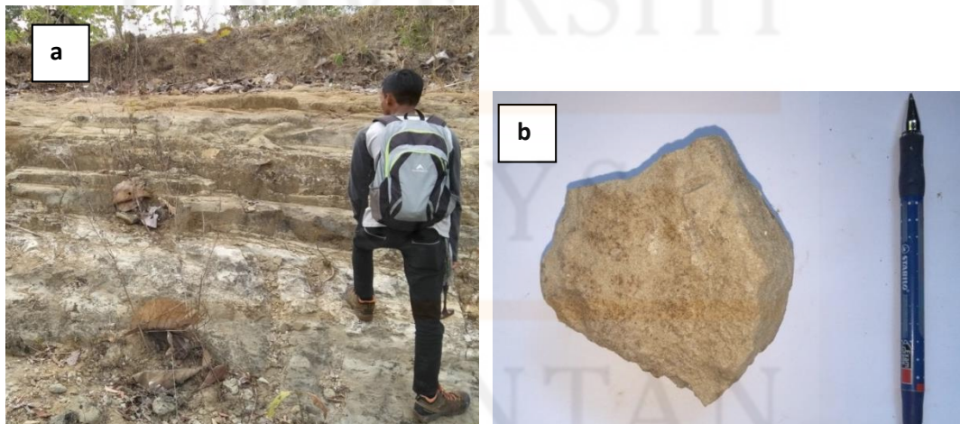
Figure 4.22: (a) Shows the outcrop of sandstone interbedded with tuffaceous siltstone and (b) hand specimen of tuffaceous siltstone. Coordinate CODE 6 NAD8C2 (S 07°52'54'', E 110°34'06'') with elevation 130 m
