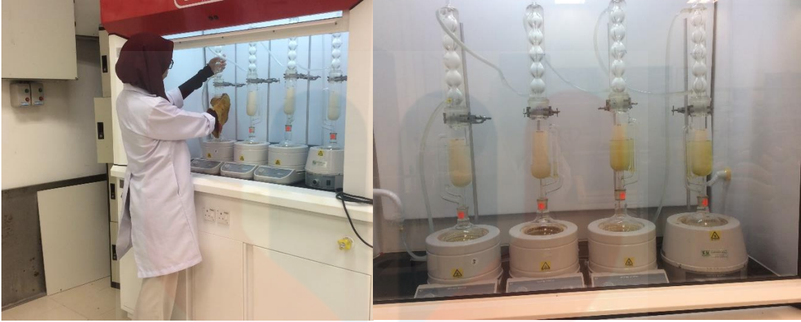
Extraction of fat by Soxhlet
