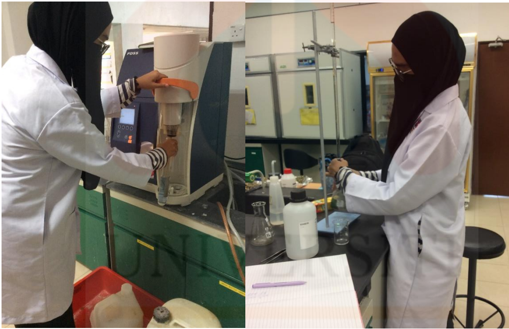
Distillation and titration process in determination of protein
