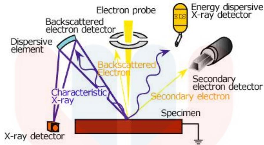
Figure 2.4: Working principle of EDX.
