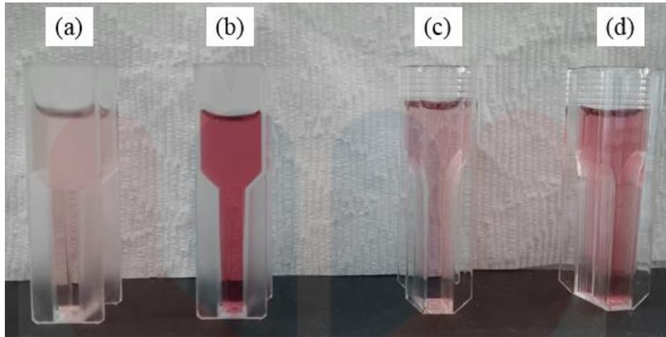
Figure 4.10: The solution from enzymatic hydrolysis which is taken its absorbance value at 510 nm. (a) Blank; (b) D-glucose standard; (c) White *D. hispida*; (d) Yellow *D. hispida*.
