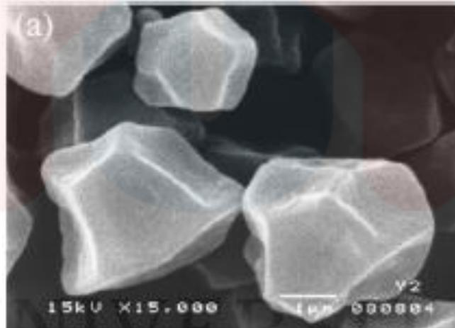
Figure 2.3: Scanning electron micrograph of native *D. hispida* starch with polyhedral shape.
