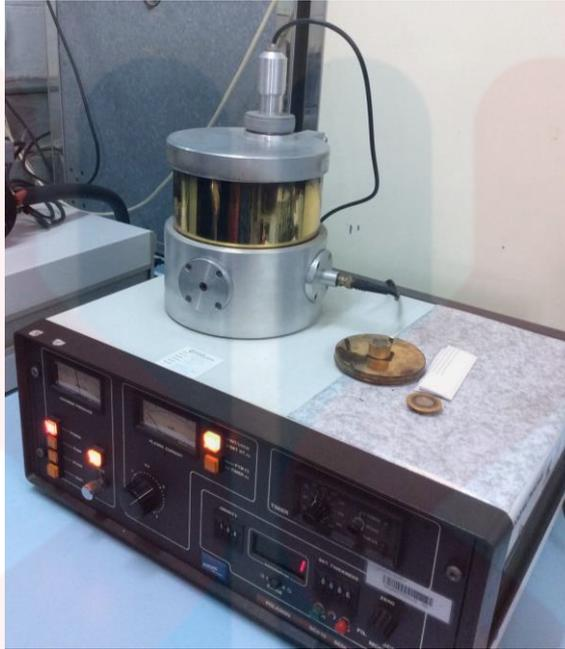
Figure 3.8: Sputtering the dried tuber cube form of two *D. hispida* cultivar with gold at low vacuum.
