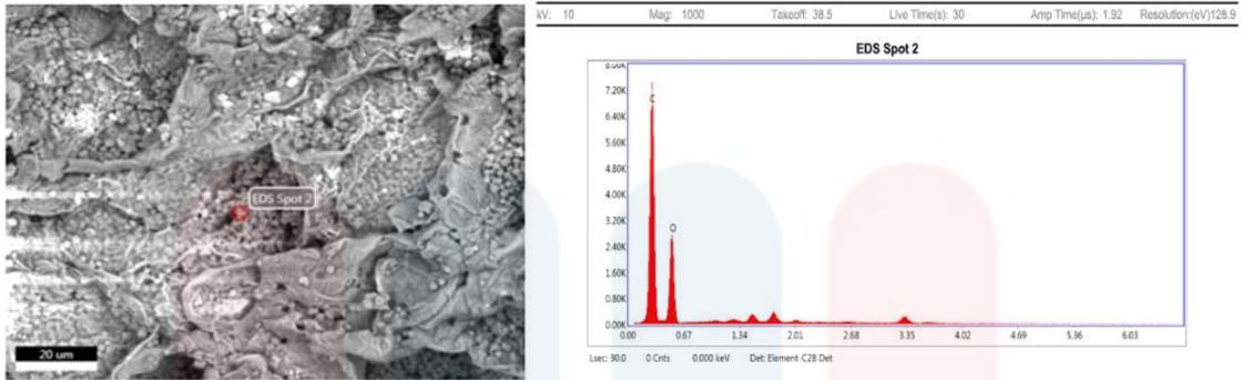
Figure 4.7: EDX graph of white *D. hispida* on the selected area, starch granule.
