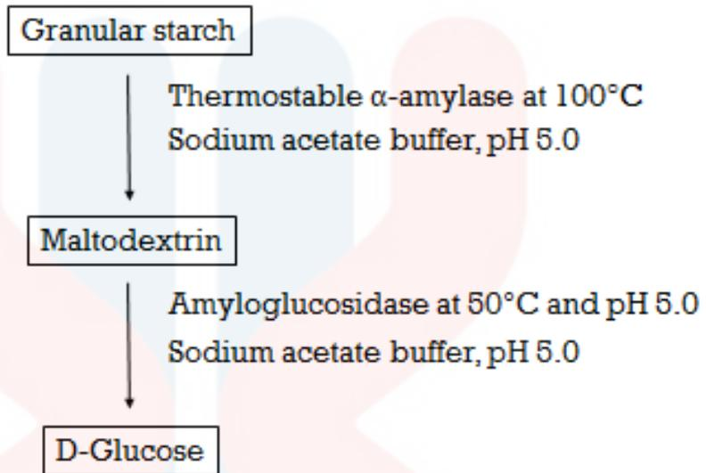
Figure 2.6: Summary of enzymatic hydrolysis of starch.
