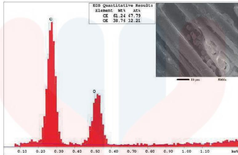
Figure 2.5: Result of the elemental analysis on starch granule exist on chestnut wood that were conducted by SEM-EDX.
