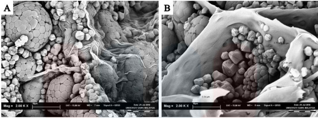
Figure 4.8: Sizing starch granule using application Cell Sens on Scanning Electron Micrograph on magnification  $\times 2000$ . (a) white *D. hispida*; (b) yellow *D. hispida*.
