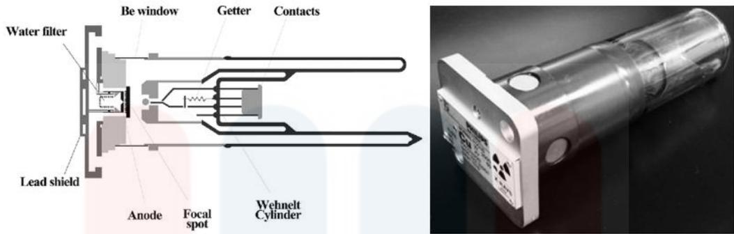
Figure 2.7: Schematic and photograph of laboratory X-ray tubes: Conventional X-ray tube type.
