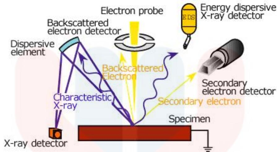
Figure 2.4: Working principle of EDX.
