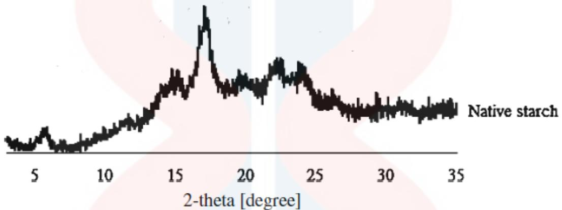
Figure 2.9: Crystallographic pattern of native starch of *D. hispida* from  $2\theta = 0^\circ$  to  $2\theta = 35^\circ$ , with highest peak shown at  $2\theta = 17.2^\circ$ .
