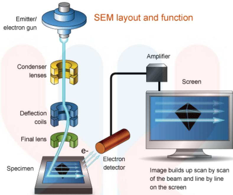
Figure 2.2: Working principle of SEM.
