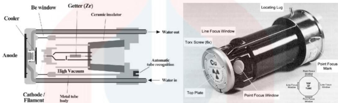
Figure 2.8: Ceramic X-ray tubes for less laborious change from line to point focus mode and vice versa.
