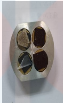
Figure 3.2: Sample preparation for SEM
