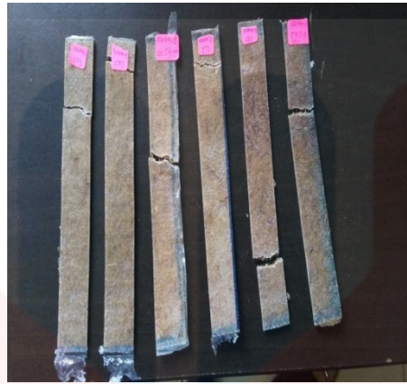
Figure 3.1: Fracture tensile samples
