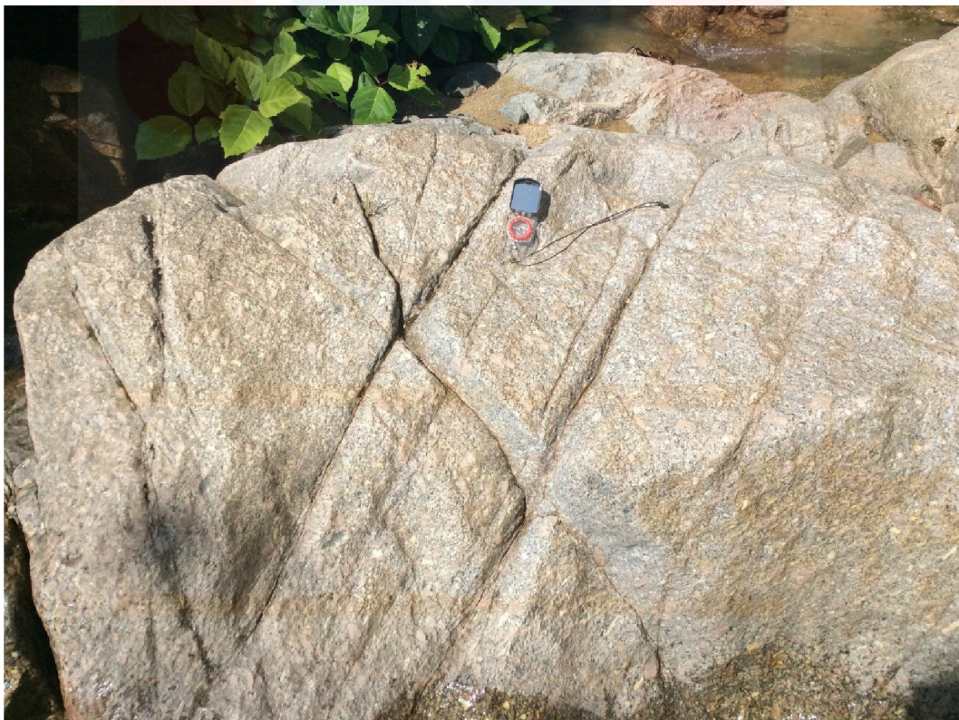
Figure 4.4.3: Conjugate shear fractures that formed from brittle deformation
