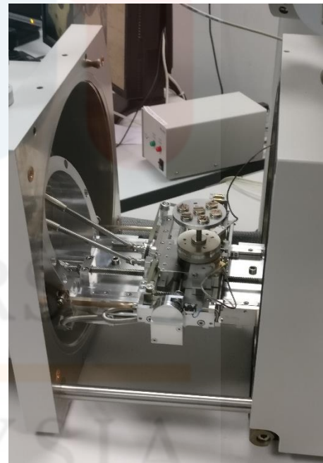
Figure A-5: Gold-coated sample before being scanned in SEM
