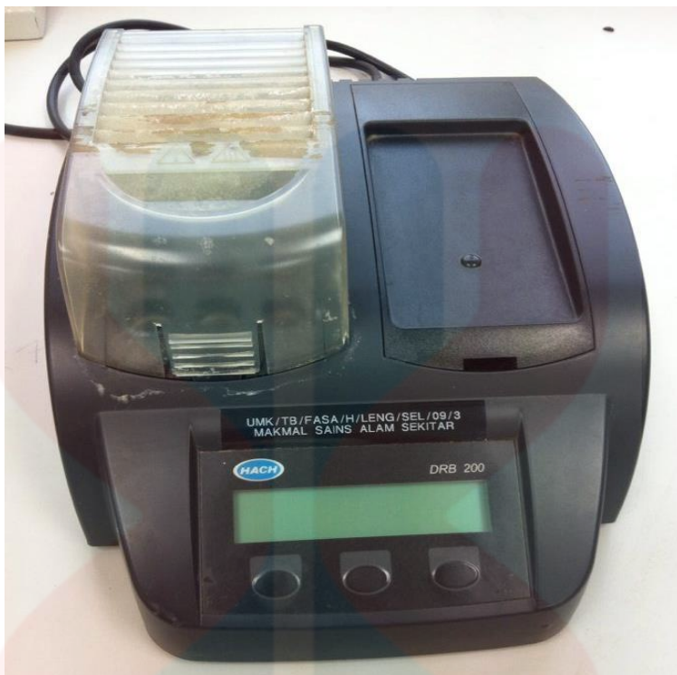
E.3: Heating water samples by DRB200 Reactor for COD reading
