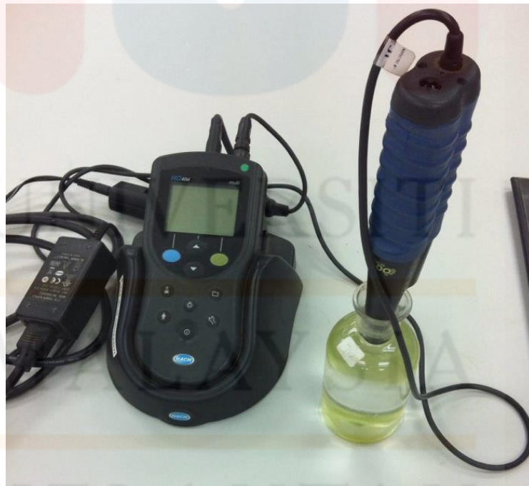
E.2: HACH HQ40d used to test BOD
