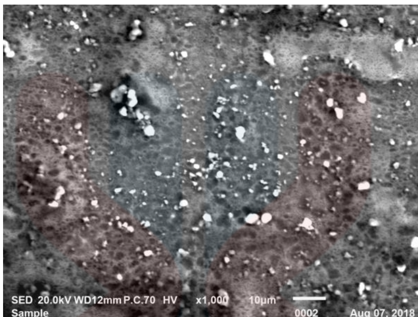
Figure 4.9: The morphology of TO/DF/ITO glass.
