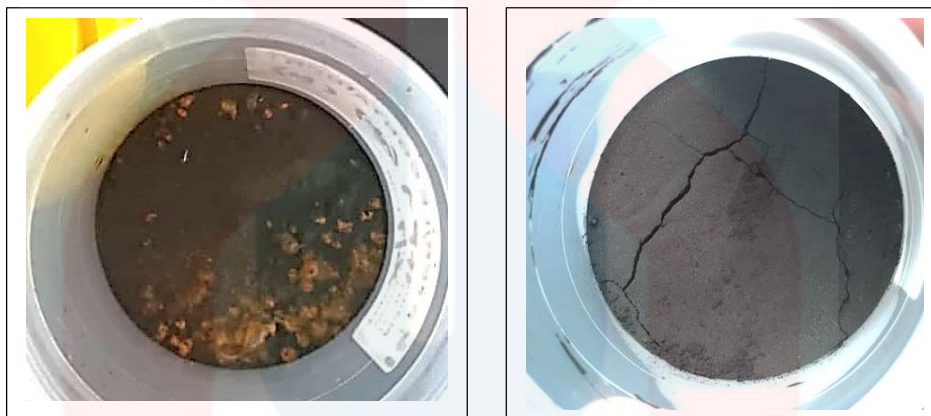
Figure 4.12.2.1: Rusted (left) and ordinary MAC (right).
