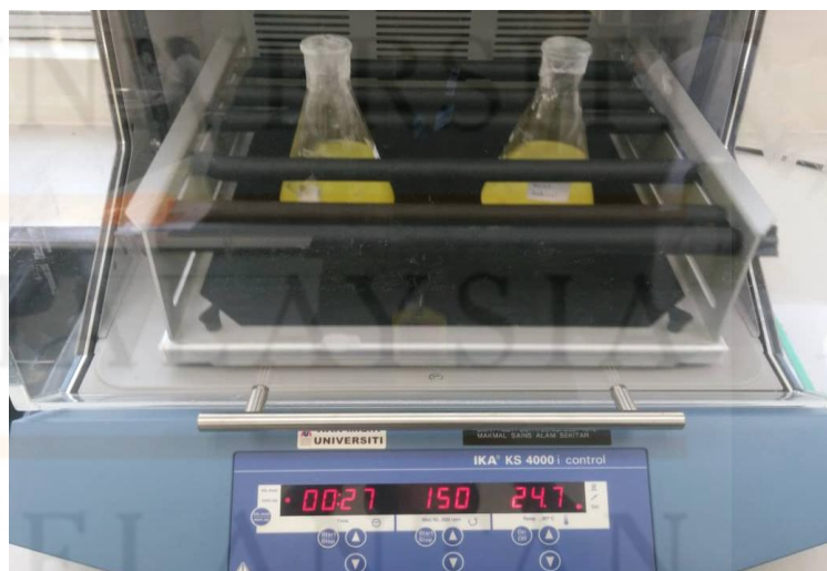
Figure 3.3: The maceration process using orbital shaker
