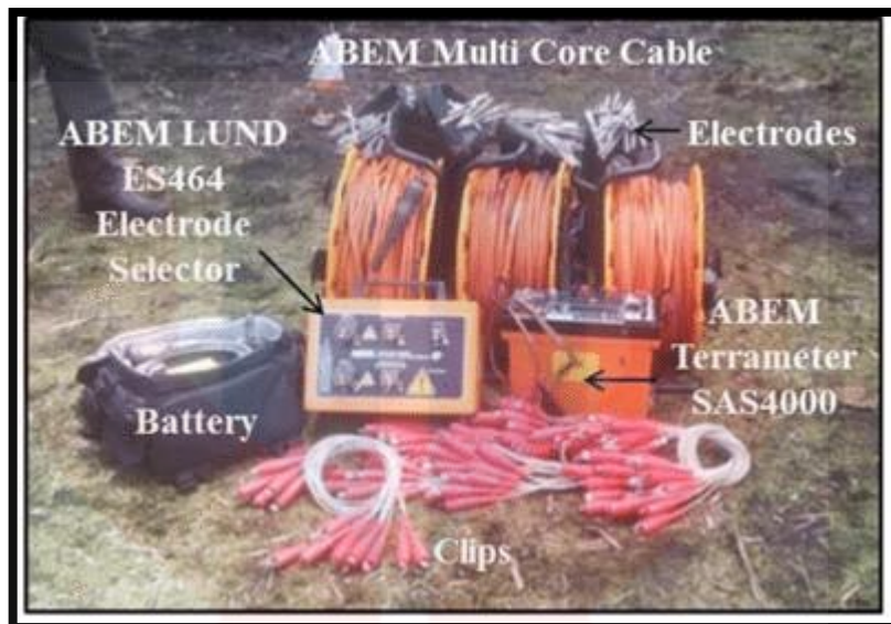
Figure 3.5: Shows a set that always come together in using Abem Terrameter.
