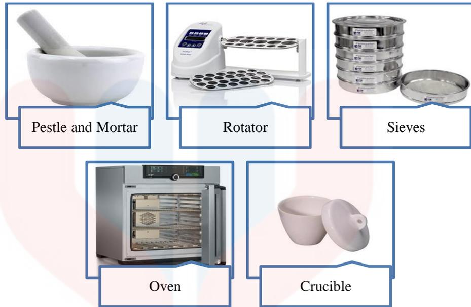
Figure 3.3: Tools for sample pulverization.
