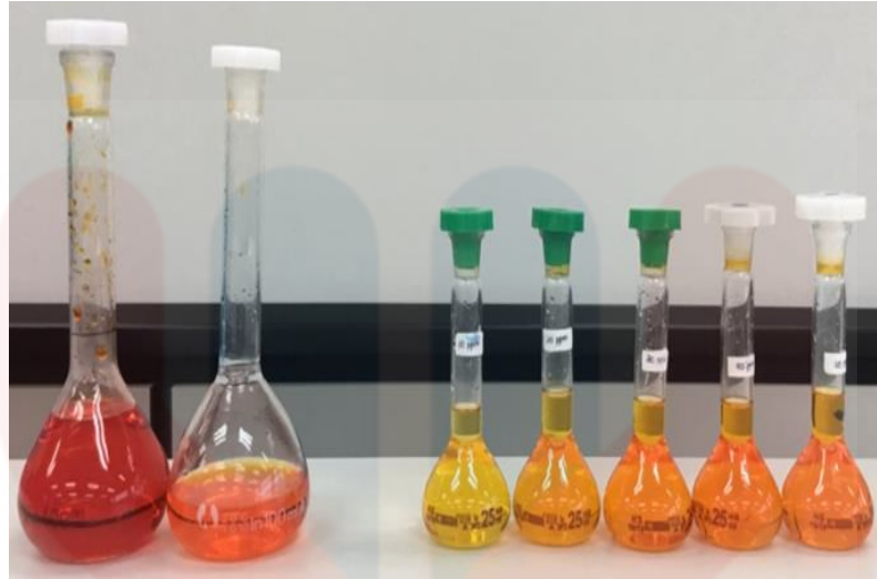
Figure B-3: The dilution of 1000 ppm of MO stock solution into different concentrations
