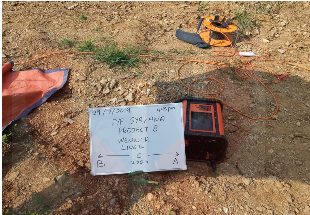
Figure 5.11: Set-up for survey line 4
