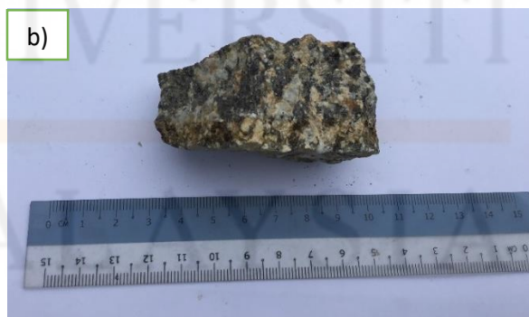
Figure 5.4: a) Outcrop of porphyritic granite at NAN S04 b) Sample of porphyritic granite
