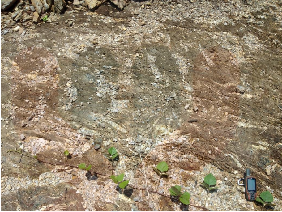
Figure 4.37: The wavy folding on metamorphic rock.
