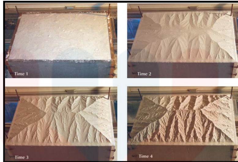
Figure 4.11: An analogy model simulates long-term evolution landform with an uplift and variable rainfall rate.
